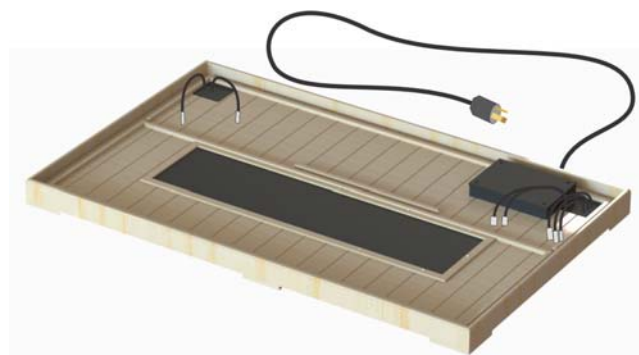
Figure 2. Laying the Floor Panel
