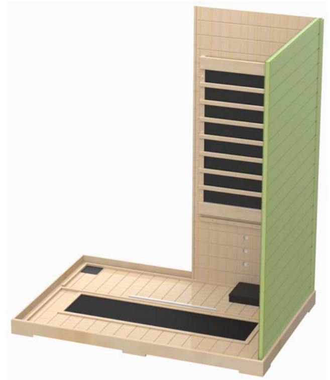
Figure 4. Installing Right Wall Section
