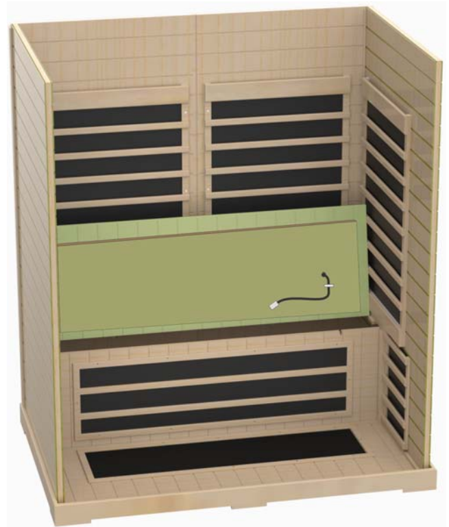
Figure 8. Installing Bench Seat
