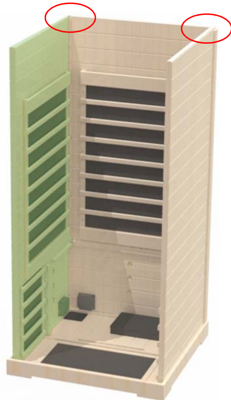
Figure 5. Installing Left Wall Section
