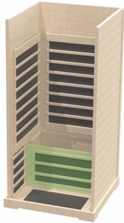
Figure 6. Installing Bench Skirt
