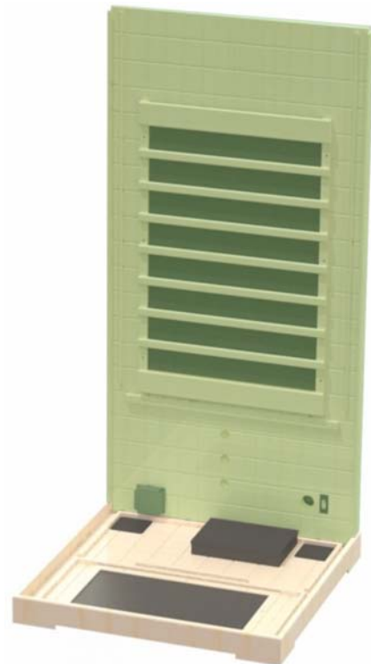
Figure 3. Installing Back Wall Section
