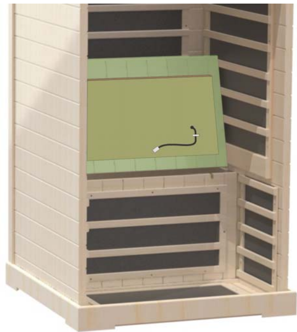
Figure 7. Installing Bench Seat
