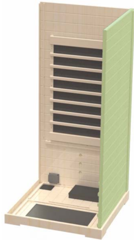
Figure 4. Installing Right Wall Section
